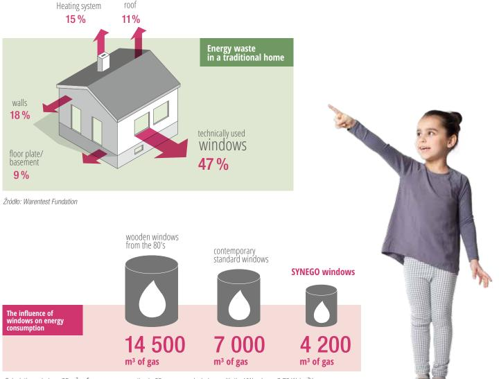
Calculation: windows 25 m<sup>2</sup> surface, gas consumption in 25 years; wood windows with the UW value = 2.79 W / m<sup>2</sup>K; standard windows with UW = 1.36 W / m<sup>2</sup>K; SYNEGO windows with a UW value = 0.66 W / m<sup>2</sup>K
