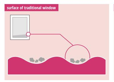
Due to the more porous structure, dirt can easily settle in cavities and is difficult to remove.
